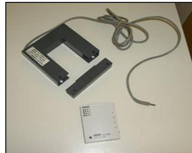
Figure 5-1: Hobo Logger and Current Transducer (CT)
