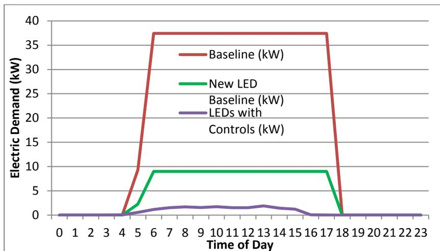
Figure 3-2: Lighting Load Profiles for Baseline, New LEDs, and LEDs with Controls (Warehouse)
