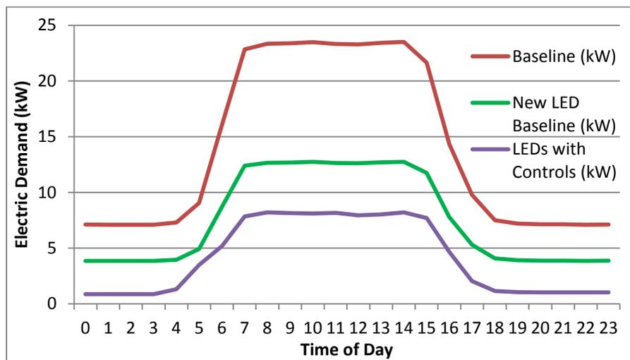
Figure 3-1: Lighting Load Profiles for Baseline, New LEDs, and LEDs with Controls (Office Areas)
