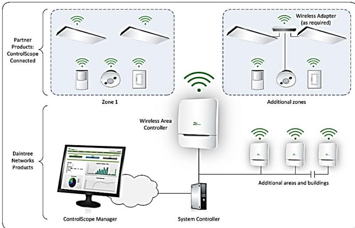
Figure 2-1: The Intelligent Lighting Controls Solution by Daintree
