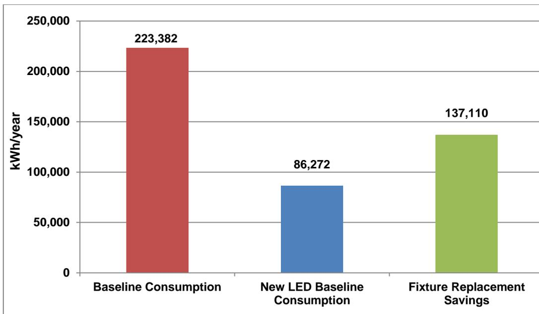
Figure 3-4: Monitored Energy Consumption and Savings for New LED Fixtures
