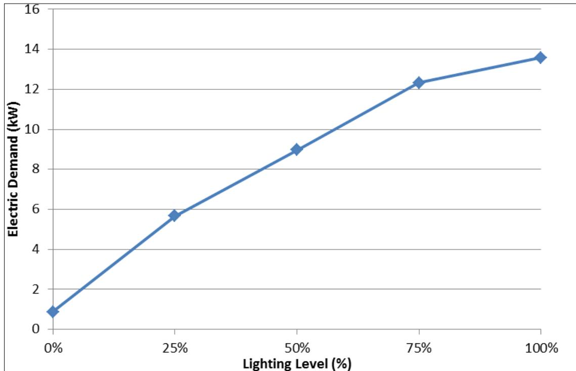
Figure 5-4: Electrical Demand at Various Dimming Levels
