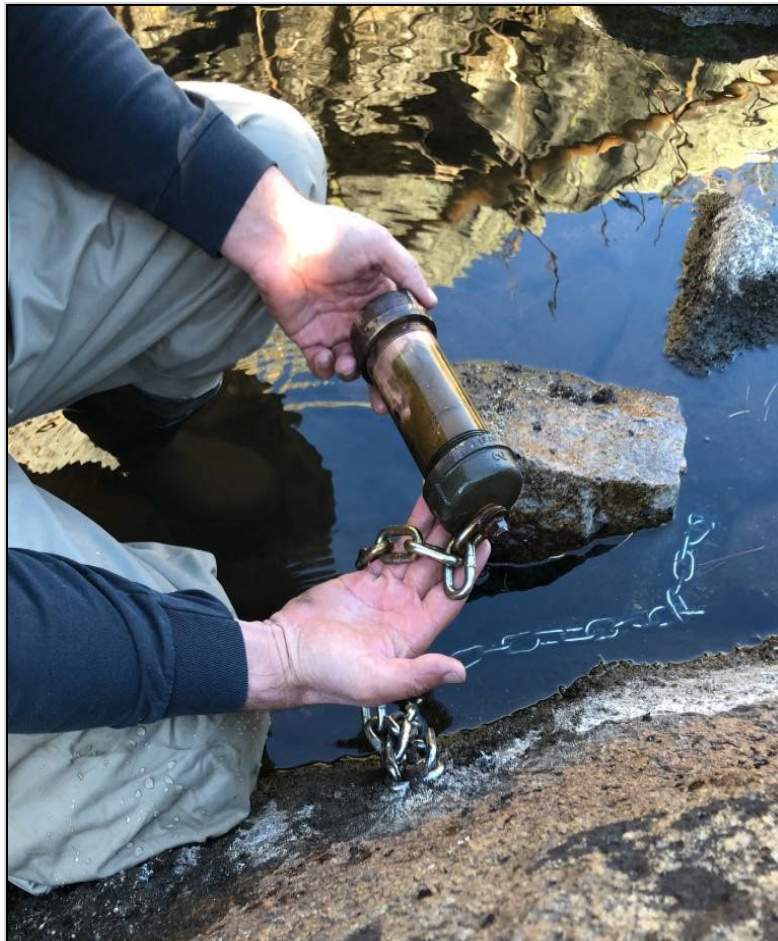
Figure 5-1. Photograph of the water temperature datalogger housing, Rubicon River below confluence of Little Rubicon River.
