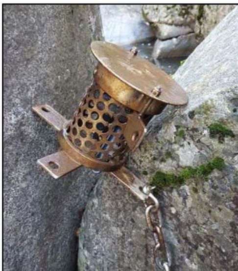
**Photo 2** – Recovered datalogger showing the standard metal housing that the HOBO dataloggers were installed in.
