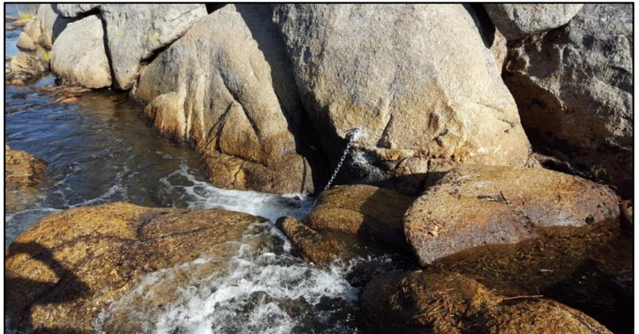
**Photo 1** – Typical install for the ONSET HOBO water temperature sensors. Sensors were installed in a metal housing secured to bedrock by heavy chain.
