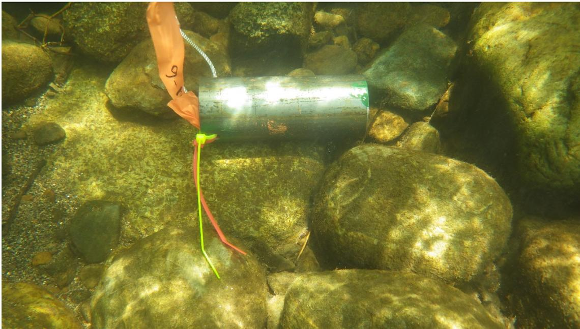
**Figure 5. Temperature Data Logger Set-up at Amphibian Monitoring Site CD-A4 (April 19, 2016)**
