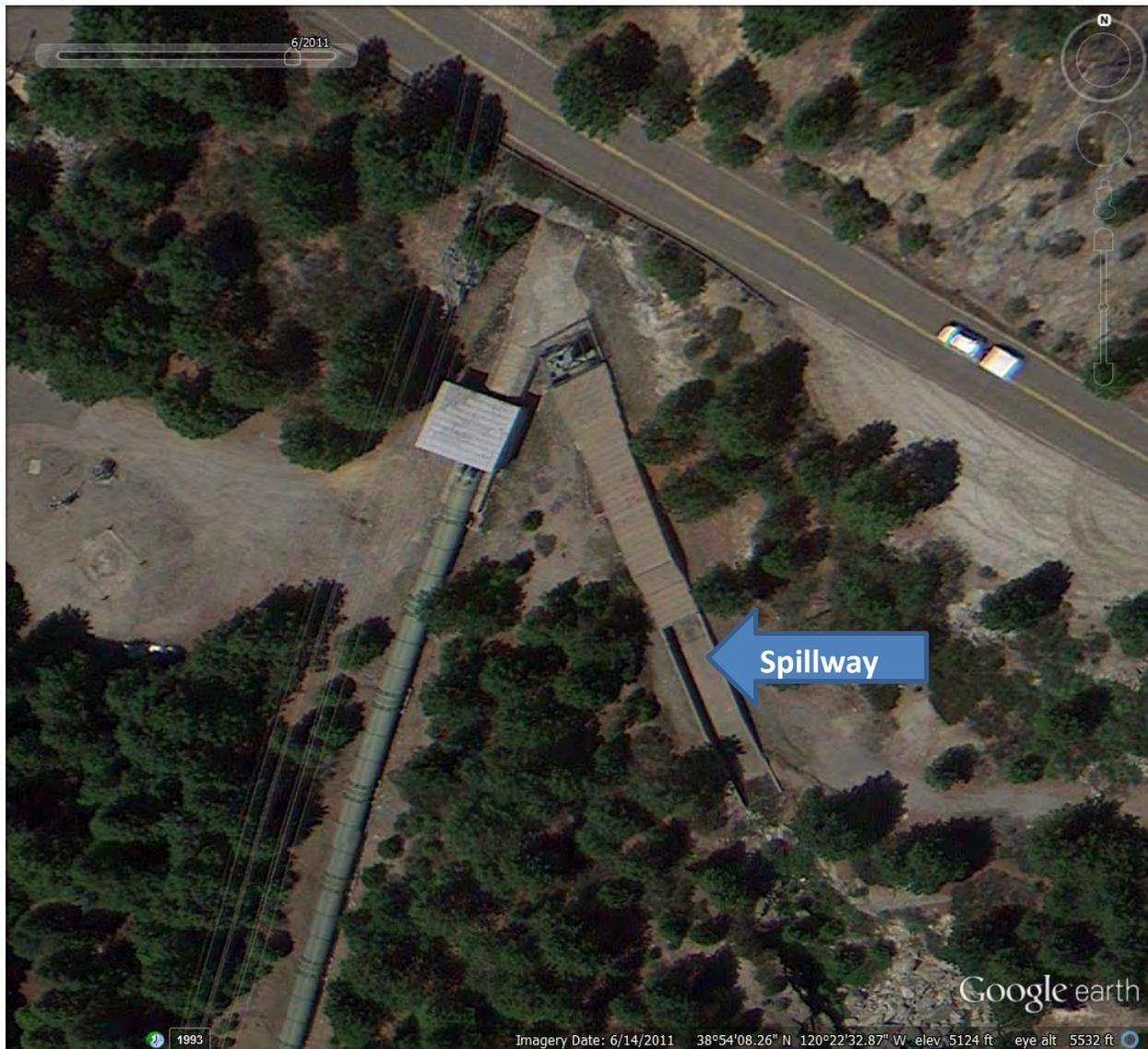
Figure 2. Flow diversion channel above Robbs Peak Powerhouse used during construction but not used as an emergency spillway.
