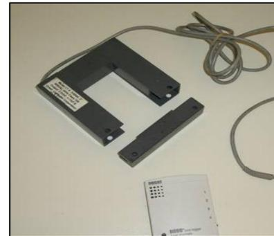
**Figure 3-1: Hobo Logger and Current Transducer (CT)**
