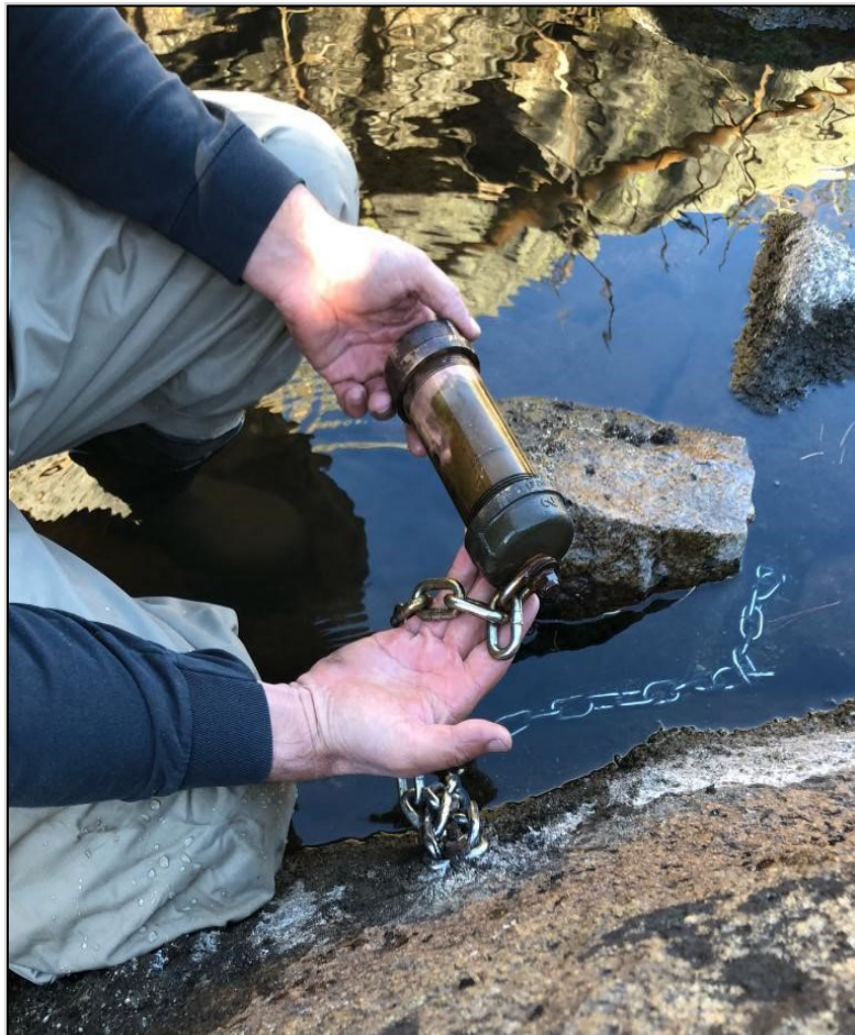
Figure 6-1. Photograph of the water temperature datalogger housing, Rubicon River below confluence of Little Rubicon River.
