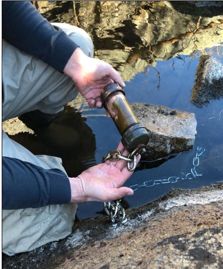
**Figure 9-1. Photograph of the water temperature datalogger housing, Rubicon River below confluence of Little Rubicon River.**
