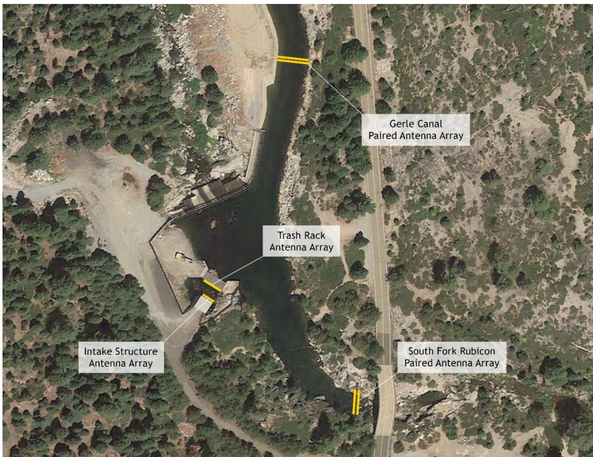
**Figure 2. Antenna configuration in Robbs Peak Forebay.**
