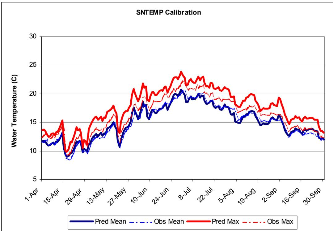
Figure 4.4-19. SNTEMP calibration results for SF American River at Mosquito Bridge (SFAR7).
