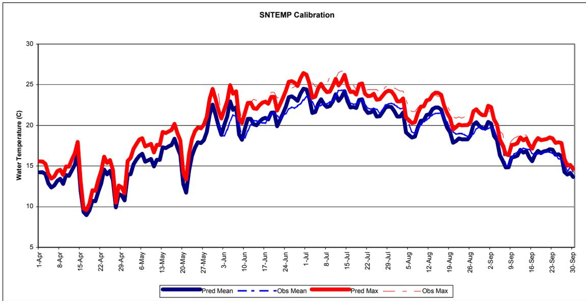
Figure 4.4-18. SNTEMP calibration results for S F American above White Rock Powerhouse (SFAR6).
