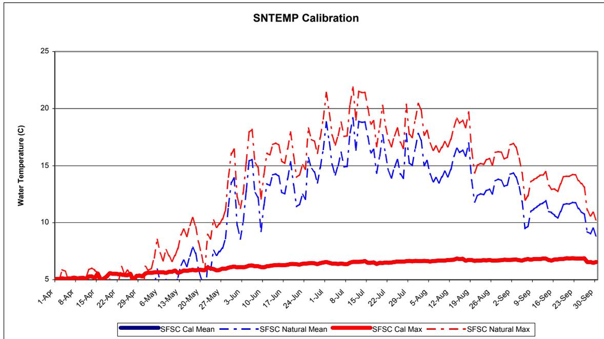
**Figure 4.4-14. SNTEMP results for South Fork Silver Creek (SFSC5 Below Ice House Dam) comparison of temperature for existing condition (calibrated) and natural flow.**
