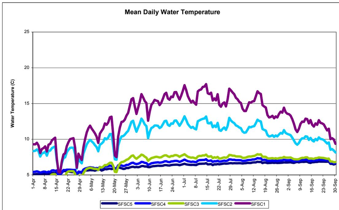
Figure 4.4-8. Predicted mean daily temperatures with a 60 cfs constant release from Ice House Reservoir.
