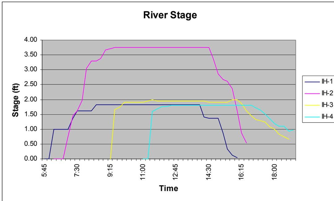
Figure I4.1-3. 15min river stage data recorded during the whitewater boating flow study.
