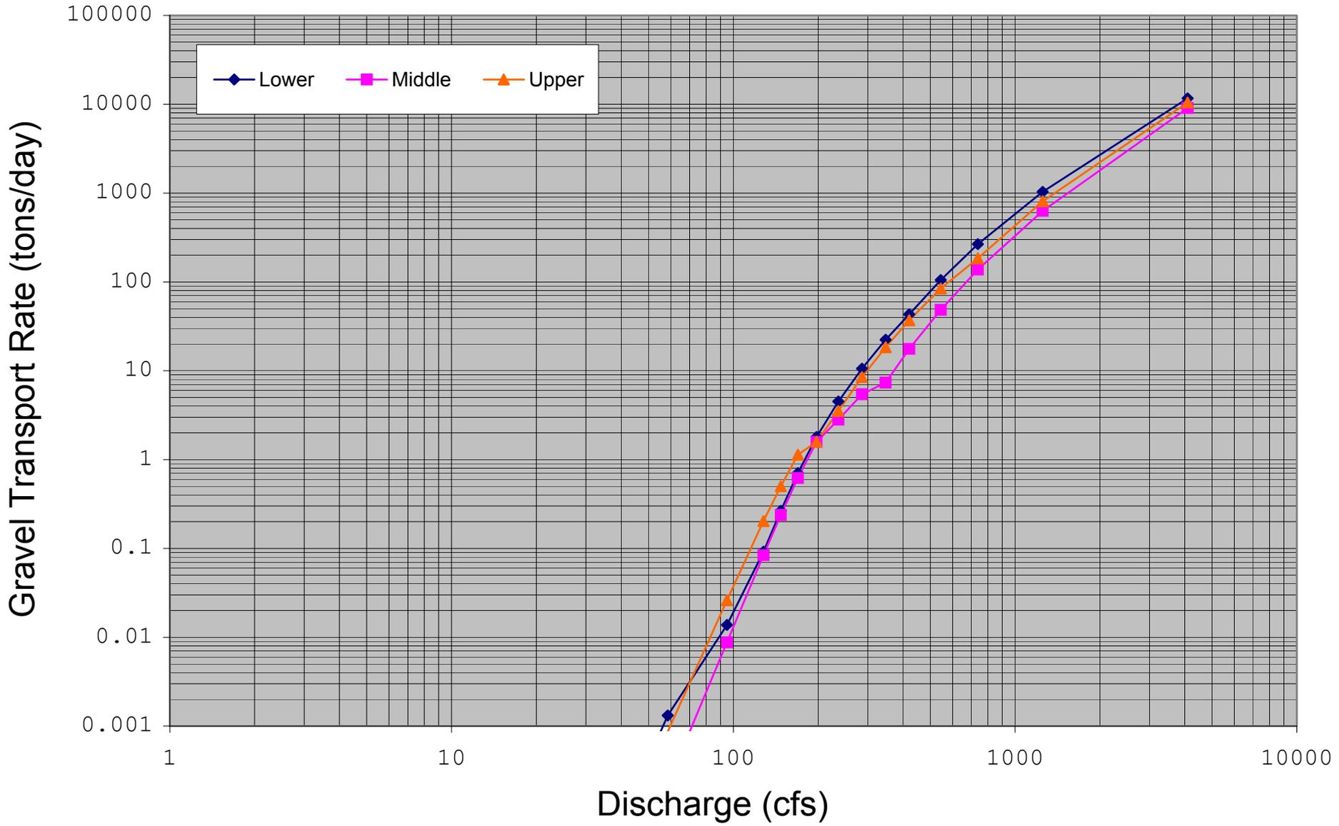
**Figure N-1: Estimated bedload transport rating curve for the Rubicon Dam Reach Site.**
