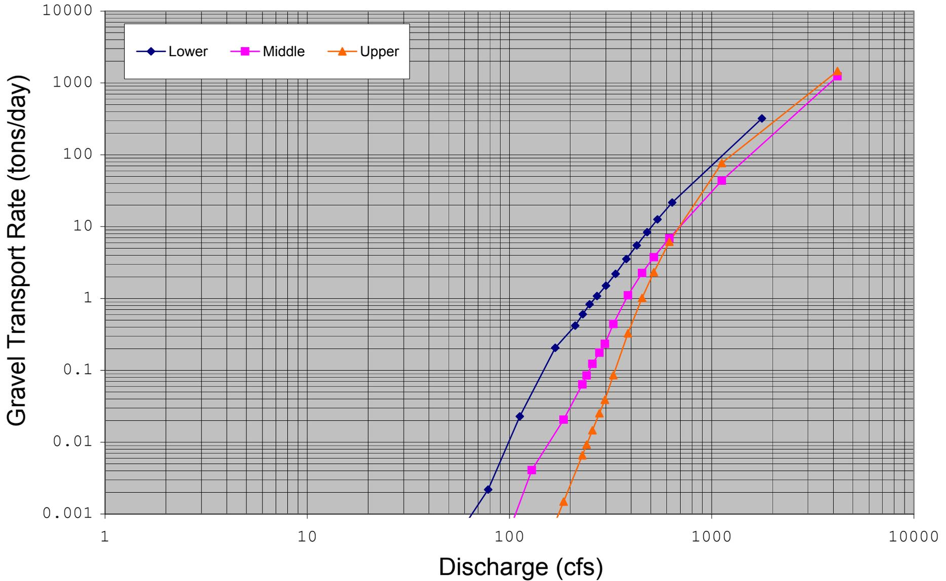
**Figure N-9: Estimated bedload transport rating curve for the Ice House Dam Reach Upper Site.**
