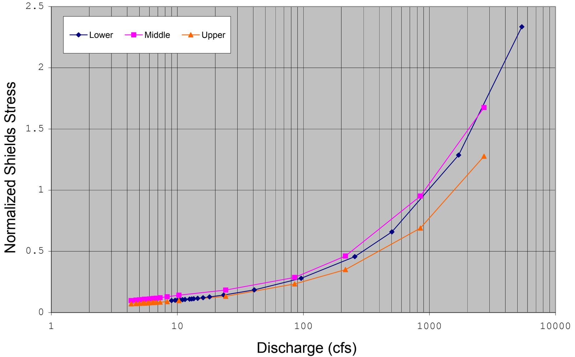
**Figure N-8: Estimated Shields stress rating curve for the Robbs Peak Dam Reach Site.**
