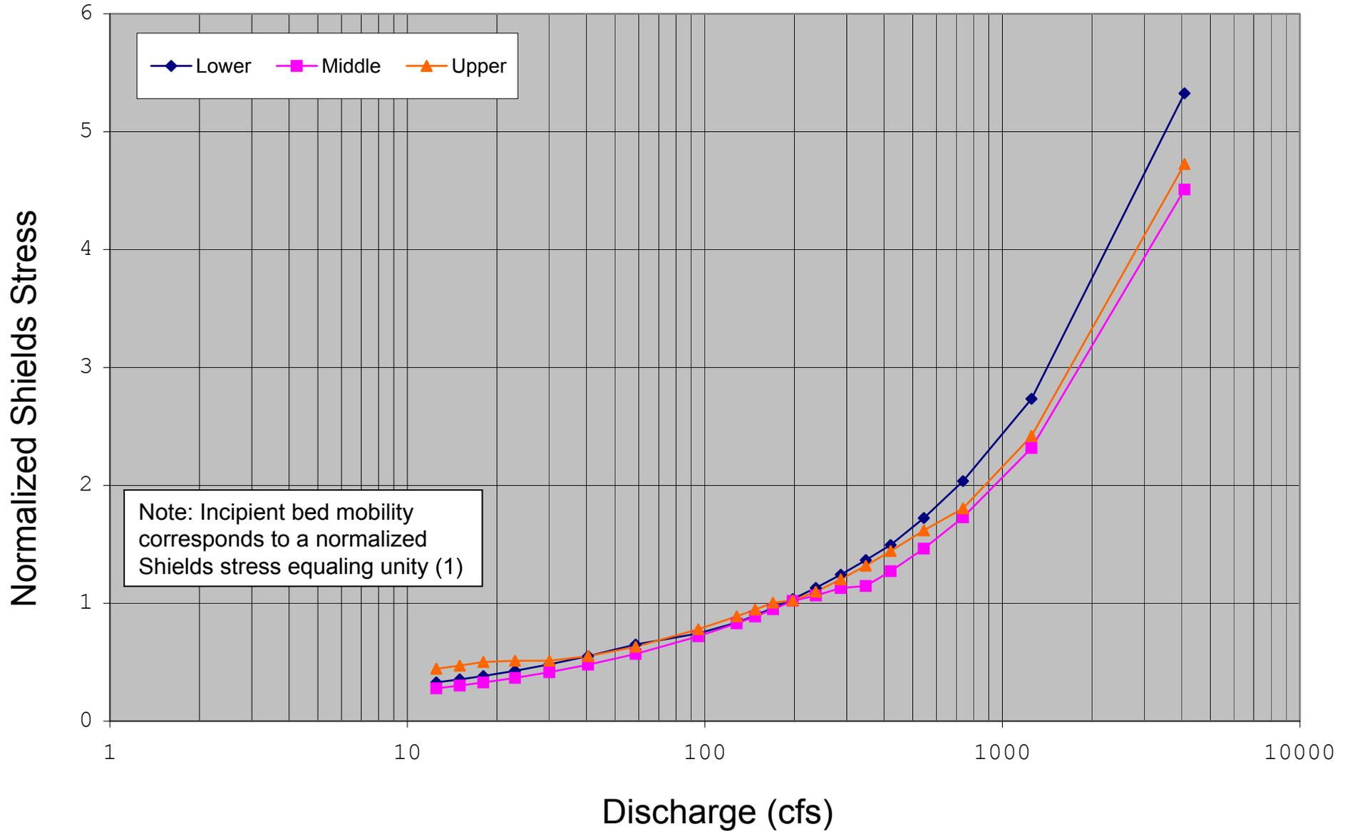
**Figure N-2: Estimated Shields stress rating curve for the Rubicon Dam Reach Site.**
