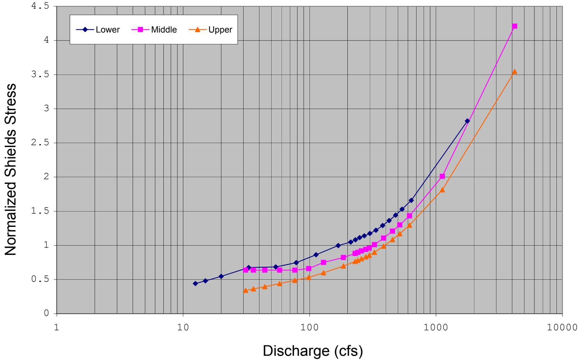
**Figure N-10: Estimated Shields stress rating curve for the Ice House Dam Reach Upper Site.**
