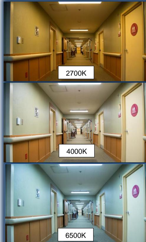
**Figure 7:** The new hallway fixtures were controlled via automatic controls for both dimming and Kelvin-changing.
