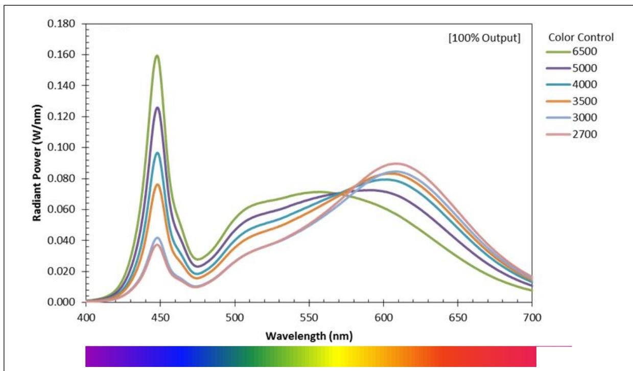
**Figure 14:** Most light sources emit different wavelengths within the visible light spectrum. The shorter wavelengths (450 nm) appear bluer and tend to have more of an impact upon people's circadian systems. The Kelvin changing fixtures used at ACC vary the spectral power distribution (SPD) by using different types of LEDs and adjusting their relative intensity levels. Source: Pacific Northwest National Laboratory.
