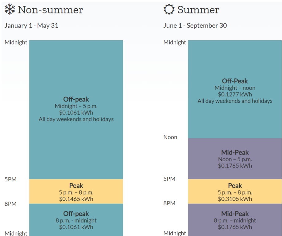
Figure 2: SMUD residential rates. On non-event days, PowerMinder optimizes operation to minimize cost.
