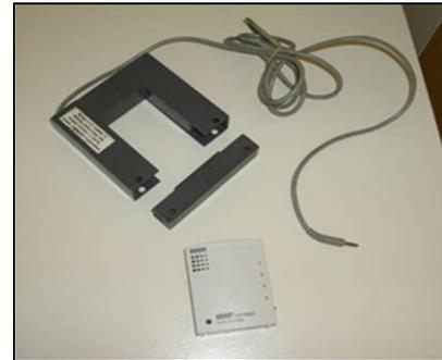
**Figure 5-1: Hobo Logger and Current Transducer (CT)**
