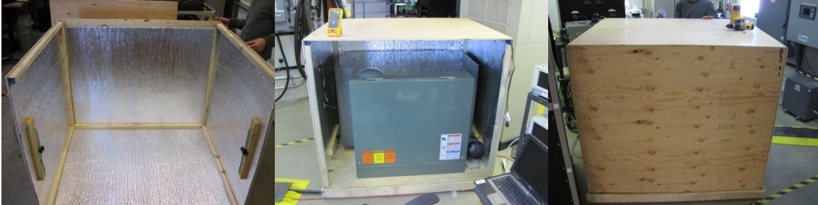
Figure 5: Photographs of Thermal Chamber Constructed for CES Testing
