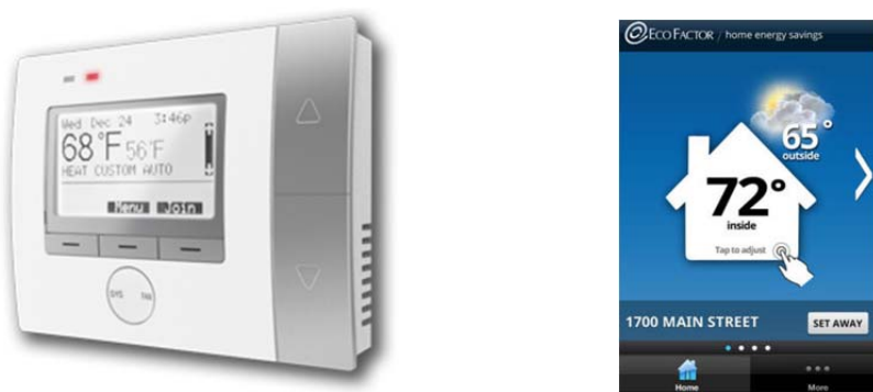
FIGURE 6. THE COMPUTIME CTW218 THERMOSTAT AND SMARTPHONE APP
