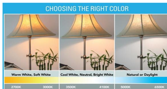
Figure 8: Ideally, people should use lights with cooler color-temperatures (5000K) in the morning and warmer tones (2700K) in the evening. For more information on this topic download our Circadian Lighting Guide via smud.org/CircadianLighting . Photo credit: Energy Star
