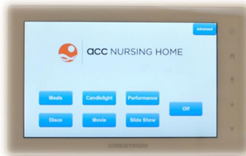
Figure 4: Incorporating a user-friendly control panel into an LED lighting system also provides several energy and user experience benefits. Building occupants are able to select from several preset lighting configurations, or “activity settings,” that vary in dimming level, lighted area, and level of direct vs. indirect light.
