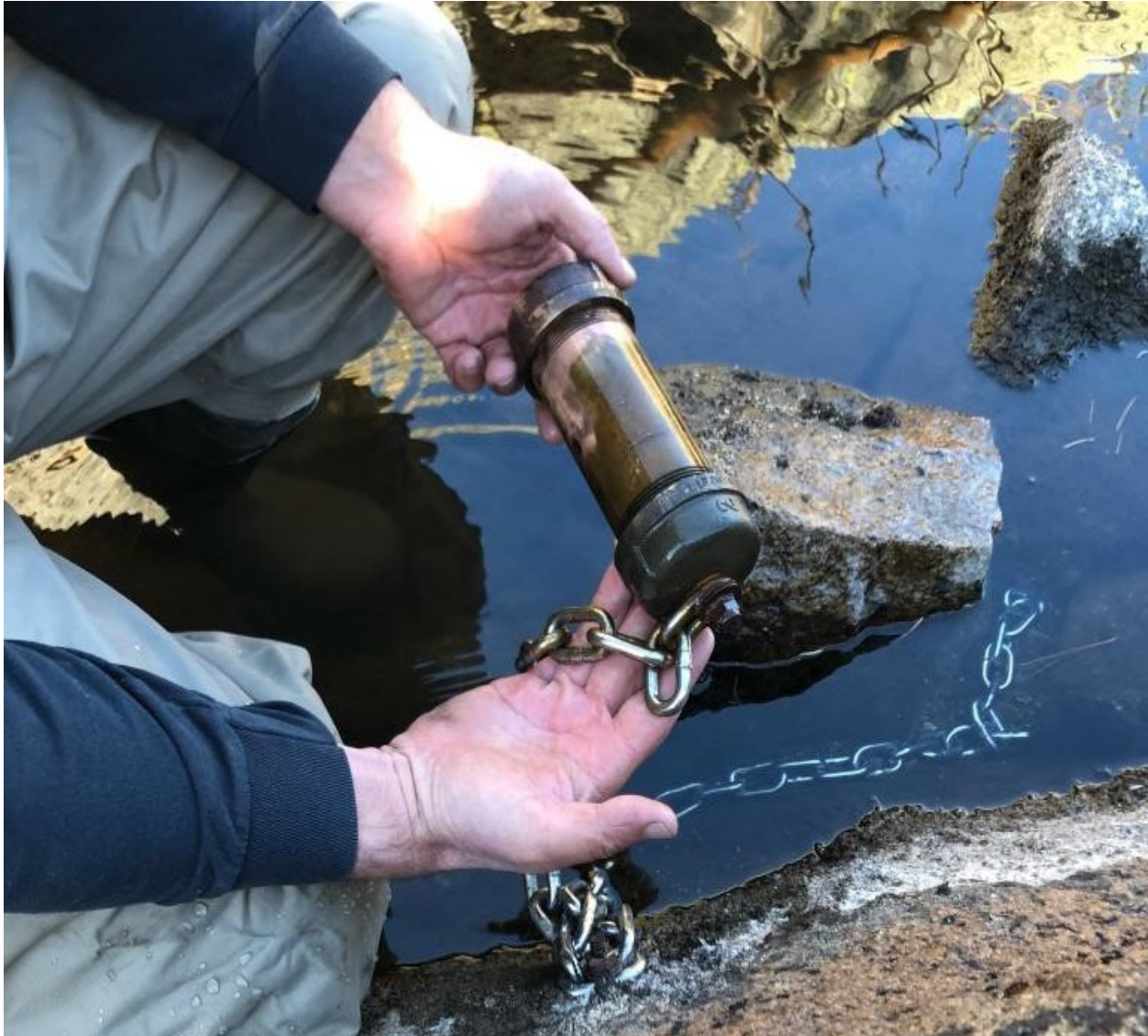
Figure 6-1. Water temperature datalogger housing, Rubicon River below confluence of Little Rubicon River.
